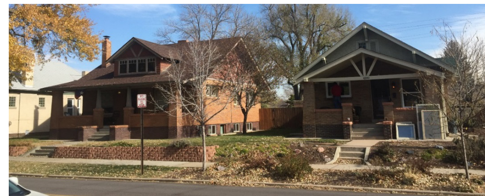
Figure 8: In the above image are two typical bungalow style buildings with 26 ft to 30 ft wide front facades. On 50 ft wide lots, which are most typical in the neighborhood, these dimensions suggest around a total of 20 ft combined side yard setback (5 ft on the narrow side, 15 ft on the larger side).
